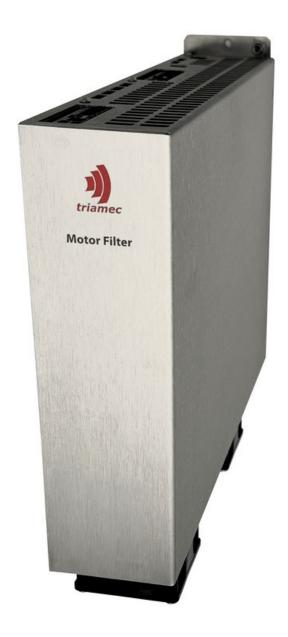
Motor-side filters of the C-series are common mode filters with minimized sinus filter stage. These filters can be used with all motor types and come as singleaxis (TFS-C) or dual-axis (TFD-C) products.
