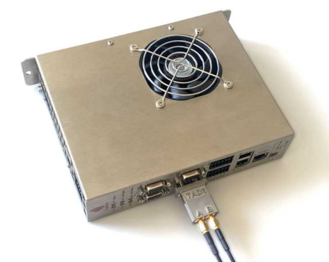
Figure 3: TAD6 mounted on Axis 0 of a TSD80
