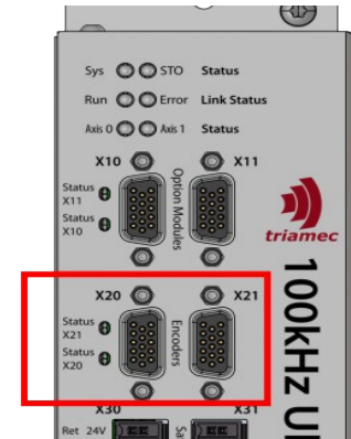
Figure 17: Encoder jack (X20,X21)
