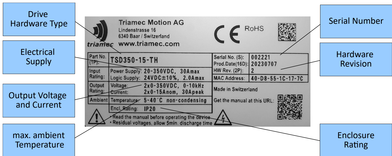
Figure 1: Nameplate of the TSD series servo drives
