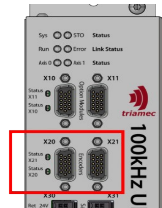
Figure 15: Encoder jack (X20,X21)
