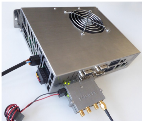
Figure 3: TAD-IEPE mounted on Axis 0 of a TSDXXX-XX-ANXX
