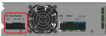
Figure 10: Brake resistor connector (X9), TSP700-10, TSP700-20
