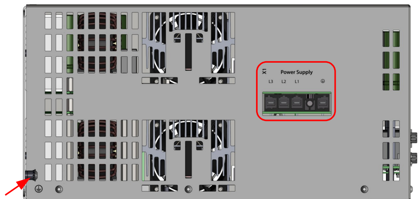
Figure 7: AC-power supply connector (X1) TSP700-40
